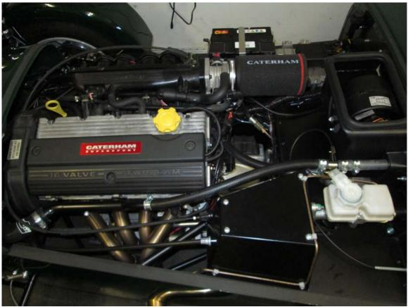
Engine: K-Series 4-cyl 135bhp 1.4L DOHC 16V
